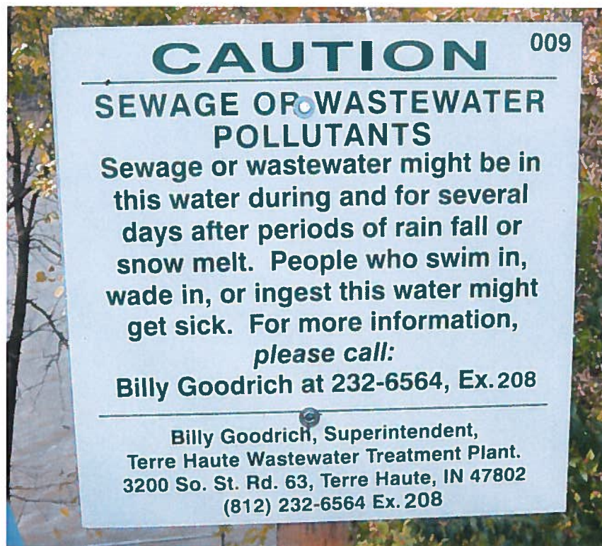
Figure 10.1 Combined Sewer Overflow Outfall Public Notification Sign
